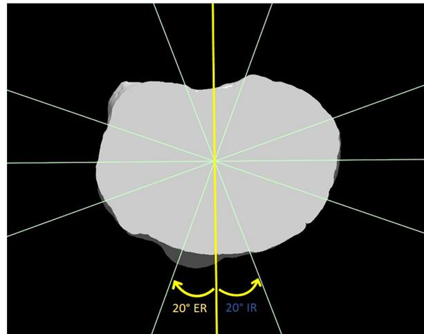
**Figure 3.** An image depicting the internal and external rotation mismatch of the tibial cutting guide.
