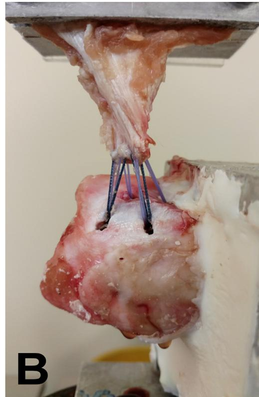
**Figure 4.** Observed mode of failure of the 2 rotator cuff tear repair suture techniques: (A) Traditional Double Row and (B) Knotless Transosseus Equivalent.
