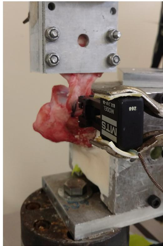
**Figure 3.** Biomechanical testing setup for comparing the 2 rotator cuff tear repair suture techniques.
