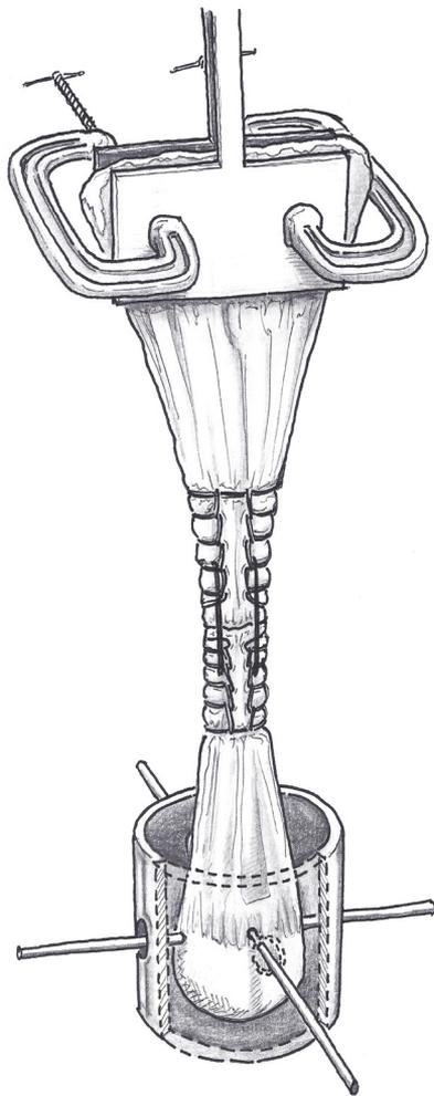
**Figure 3.** Depiction of study repair mounted in MTS machine as setup for this study. Proximally, a soft tissue freeze clamp is affixed at the level of the musculotendinous junction. Distally, two orthogonally placed Steinmann pins pass through the calcaneus bone block and are secured in a fenestrated aluminum housing.
